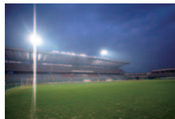
Conventional CCD Sensor (vertical smear)
